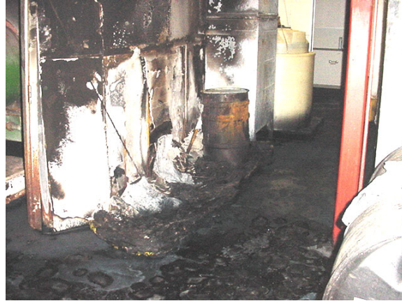
Figure 3. Thermogram/photo showing the heated sodium hydrosulfite in a 32 gallon drum.
